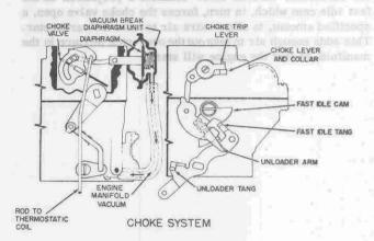
The choke system on the model H carburetor for 1962 is fully automatic. A separate choke will be used in each carburetor and will operate independently.
