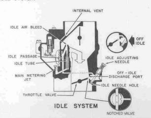
Operation is basically the same as on previous models except for the following changes which were made for improved idle operation and low speed performance.
